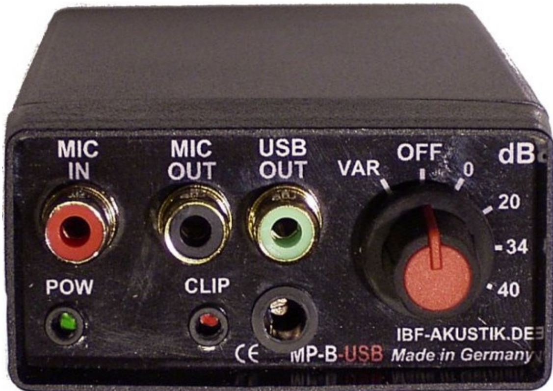
MP - B - USB (has direct USB connection & built in sound card)
